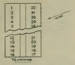
There seems no doubt that the temperatures as a whole were in excess of the intended average of 650° C. The causes of this variation are, partly, as expressed above, the situation of the setting and the design of the combustion chambers and partly the nature of the fuel gas. This gas was an imperfect mixture of rich coal gas and producer gas and layering must have occurred from time to time in the holder supplying the burners.
